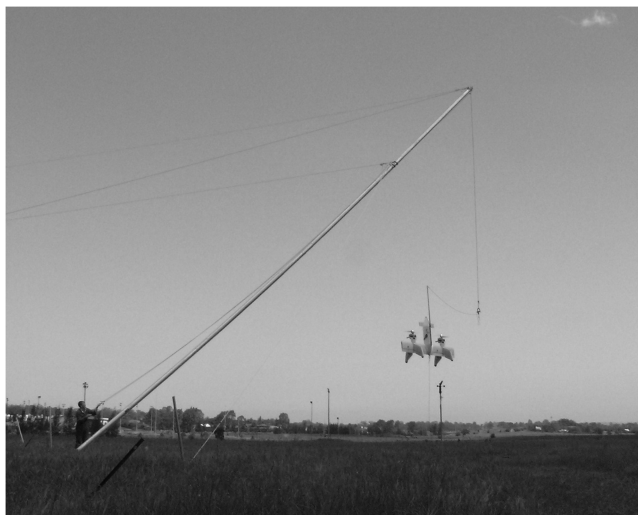
Fig. 17 Tether test rig with T-wing flying below; both tethers are slack; first author is to the left, managing the tether rope.
