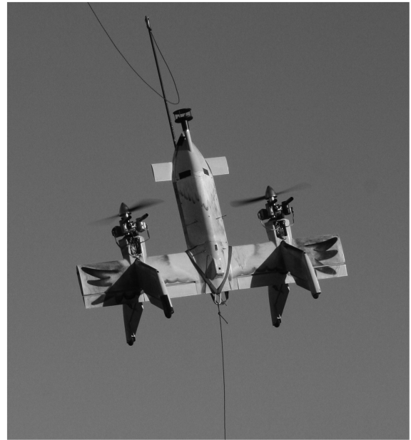
Fig. 9 Vehicle in hover-mode flight in wind with ultrasonic wind sensor on nose.
